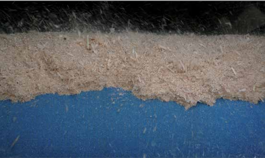
1. CONDUCTO process belts for drying wood shavings 2. PAD seam 3. CONDUCTO 5065
