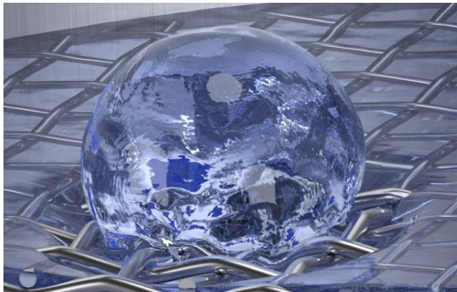
Picture 1: Visualization of a bubble-break-through in a Bubble point test.
