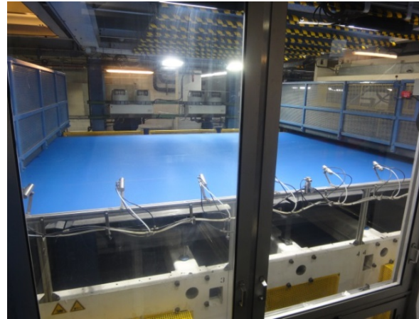
Picture 2: The laydown belt CONDUCTIVE® 7701 made by GKD – GEBR. KUFFERATH AG meets the requirements from Multitexx concerning air permeability and the uniformity perfectly due to its structure.
