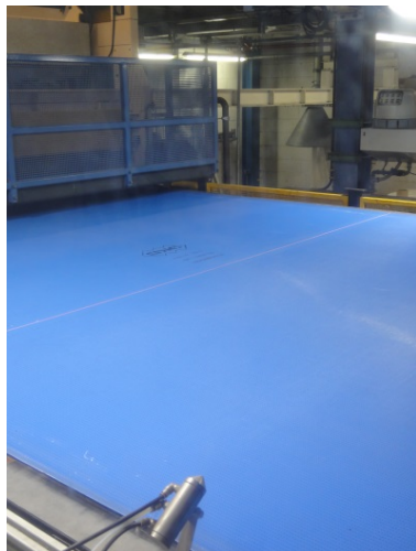
Picture 3: The circulating laydown belt type CONDUCTIVE® made by GKD – GEBR. KUFFERATH AG is almost 33 metres long and 3,80 metres wide.
