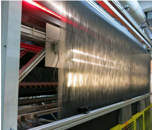
Picture 6: The visual control of the filaments at the Reicofil line ensures accurate quality.
