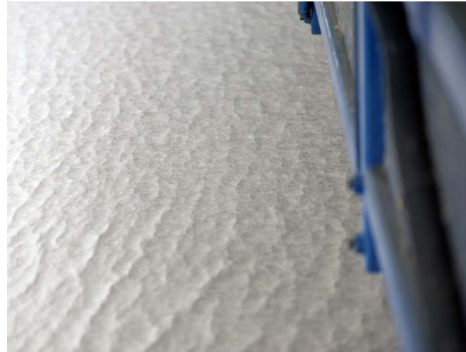
Picture 7: The CONDUCTIVE® 7701 made by GKD – GEBR. KUFFERATH AG transports the filaments on the wire mesh belt for the hardening in the calender.
