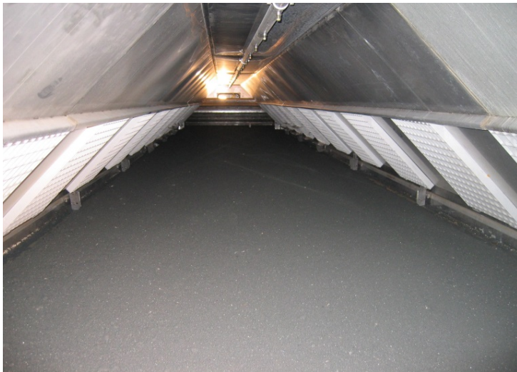
Picture 3: Air permeable and with high lateral and dimensional stability, dryer belts from GKD guarantee sewage sludge drying in high or low temperature dryers that is just as cost-saving as it is environmentally friendly.
