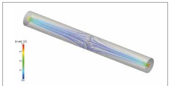
CFD-calculated fluid path while back-pulsing
