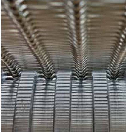
Picture 1 Self-tracking belt. With flexible cables as warp wires in MD and „V-crimped“ solid wires in CD. Picture 2 Edge treatment. Weft wires are secured by welding two or three wire ends together. This avoids unraveling and enables a high wear-resistance of the edges. Picture 3 Looped pin seam. Easy and economic belt installation with a solid pin wire.
