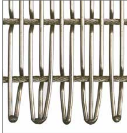
Picture 1 Self-tracking belt. With flexible cables as warp wires in MD and „V-crimped“ solid wires in CD. Picture 2 Edge treatment. Weft wires are secured by welding two or three wire ends together. This avoids unraveling and enables a high wear-resistance of the edges. Picture 3 Looped pin seam. Easy and economic belt installation with a solid pin wire.
