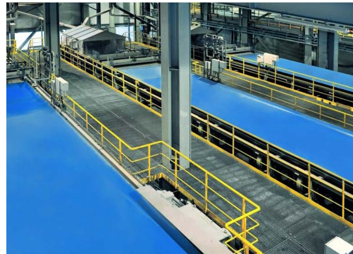
Picture 4: The VACUBELT® 2015 filter belt from GKD has been the globally established standard in the field of FGDP gypsum dewatering for many years.
