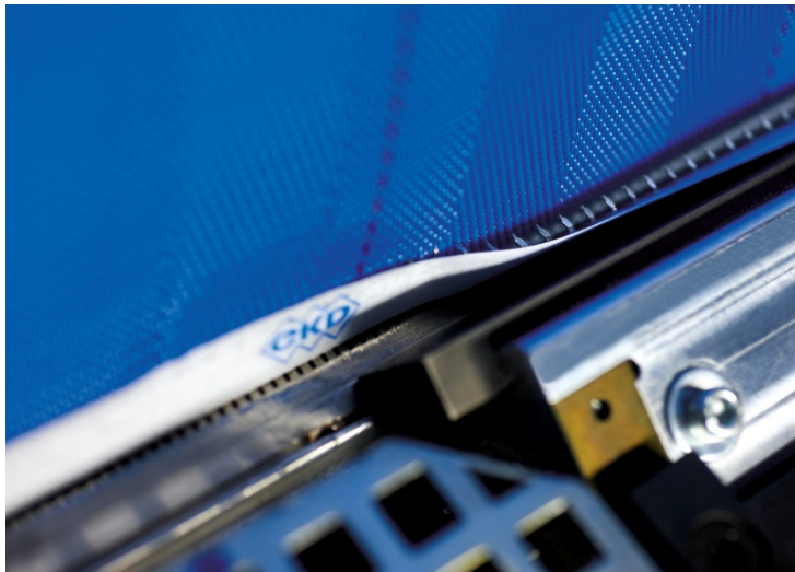
Picture 1: Filler threads are inserted into the PAD seam from GKD before the clamps are closed thereby further lowering the risk of particle penetration.
