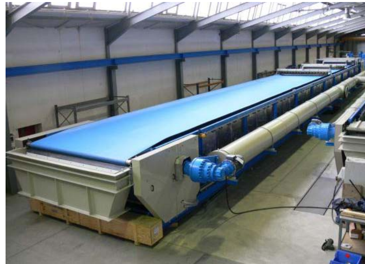
Picture 2: Single-ply vacuum filter belts of the type VACUBELT® from GKD are specifically designed for particular processes and thermally treated for the dewatering of phosphogypsum.
