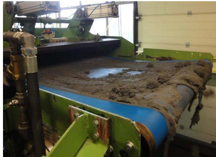
Picture 6: In cooling lubricant filtration, the robust VACUBELT® 3354 filter belt from GKD reliably retains swarf and particles abraded from the grinding wheel.
