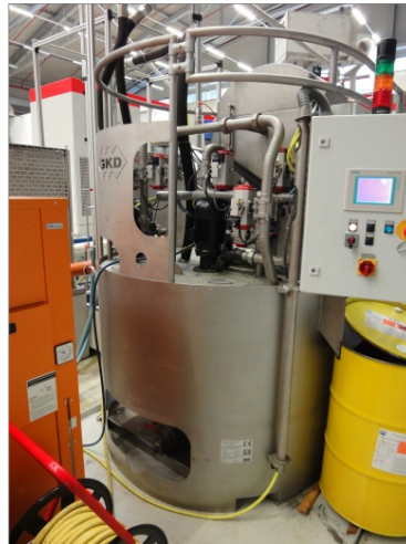
Picture 7: With the required filtration level of \leq 5 \mu\text{m} the filtration rate is 200 litres per minute.
