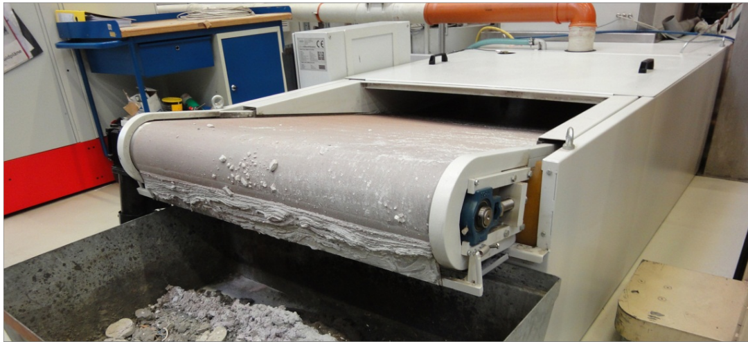
Picture 8: Self-cleaning MAXFLOW belt filter for particle separation \leq 40 \mu\text{m} .
