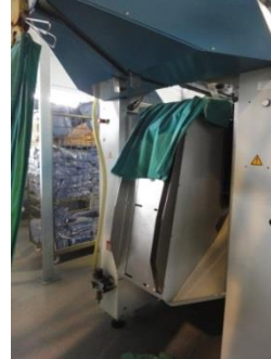
Picture 10-12: The laundry is hung per hand on the clips or hangers of the conveyor system and passes in sequence through a range of ironers where they are also directly folded.
