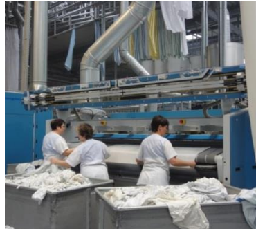
Picture 10-12: The laundry is hung per hand on the clips or hangers of the conveyor system and passes in sequence through a range of ironers where they are also directly folded.
