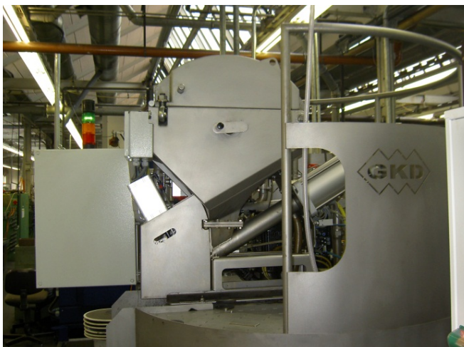
Picture 3: The compact unit with filter head and briquetting unit in action at Gühring.
