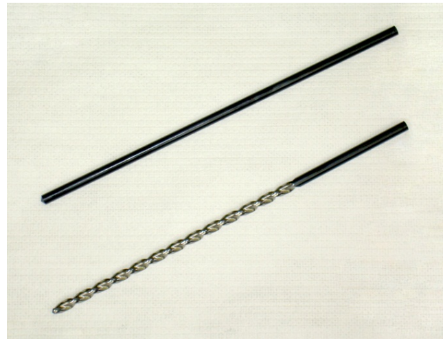
Picture 6: The steel rod before and after the conditioning by Gühring.
