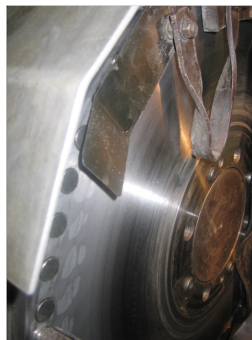
Picture 7: During the double face grinding process the cylinders are ground to the specified length on both sides by rotating grinding disks.
