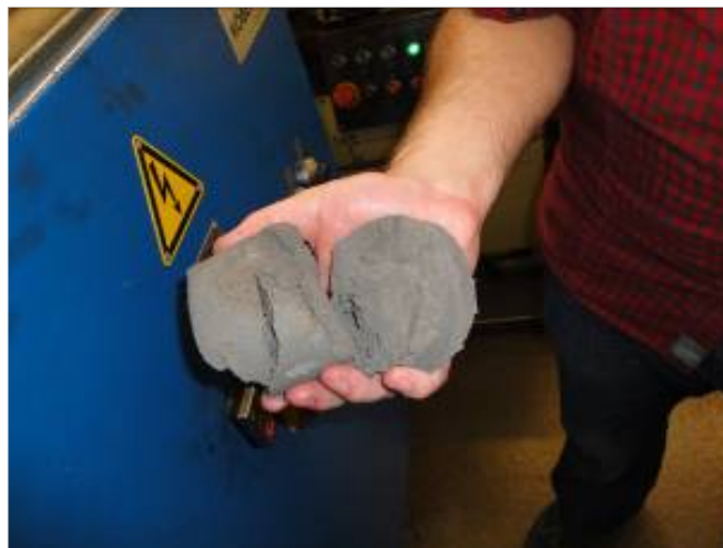
Picture 9: The MAXFLOW system, designed for machining processes, combines filtration and briquetting in one unit.
