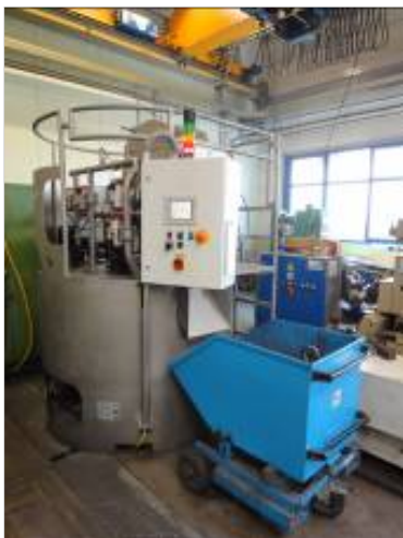
Picture 8: In order to improve the production process, the MAXFLOW compact filtration system is used for the length grinding process.
