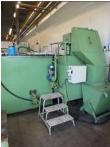
Picture 2+3: For the filtration of the cooling lubricant emulsion KRS-MARABU uses the belt filter with magnetic separator.
