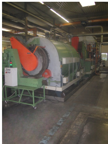
Picture 5: After deburring and cleaning, the blanks are tempered to final hardness in the tempering furnace.
