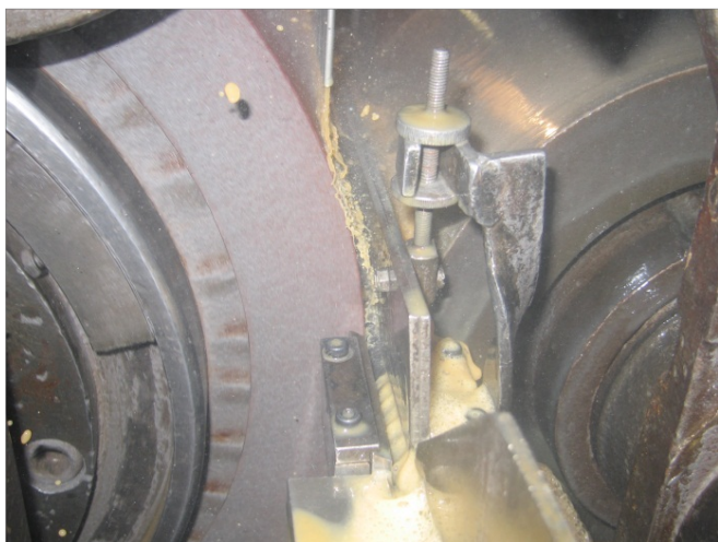
Picture 6: During the centre-less diameter grinding the parts are shaped into the required diameter with tolerances of 2 -4 \mu\text{m} .
