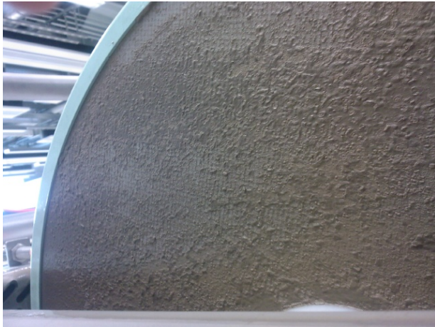
Picture 9: Automatic backwashing detaches the filter cake of milling waste.
