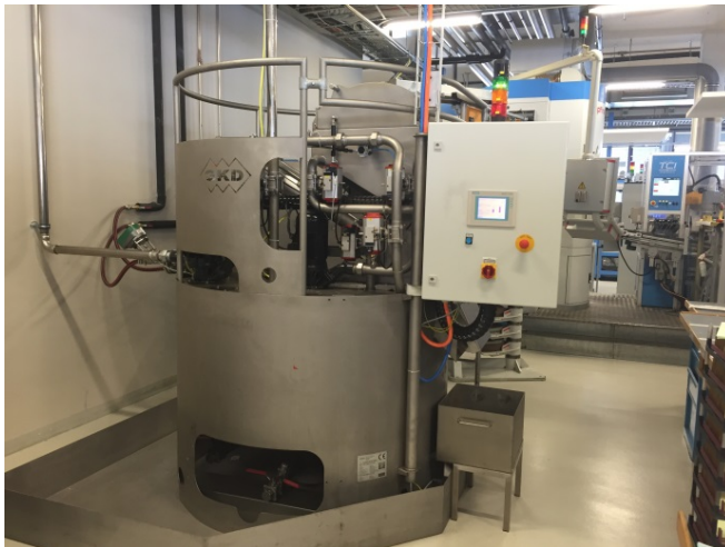
Picture 7: The compact filter system MAXFLOW CS 1000 combines filtration and Filtration und briquetting in one plant.
