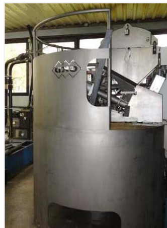
Picture 5: Jores trusts the MAXFLOW compact filter system for the filtration of the cooling lubricant.
