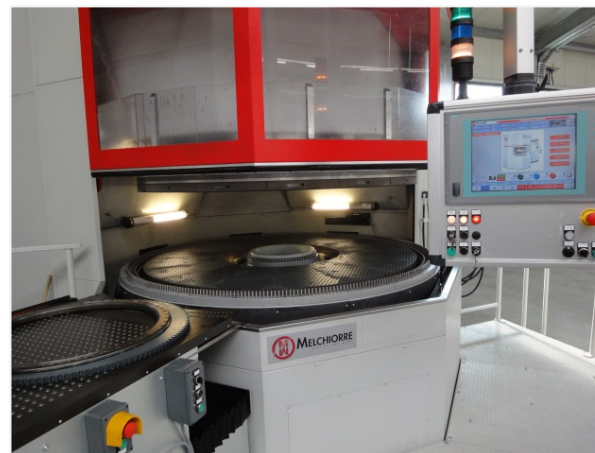
Picture 6: What currently ranks as the world's largest precision grinding machine has been put into operation at the Jores grindery for double-sided face grinding in batch process.
