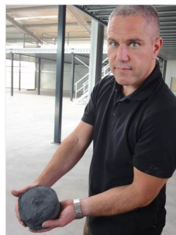
Picture 11-12: The pressing unit integrated into the MAXFLOW compresses the residues into briquets and ejects them into collection bins.
