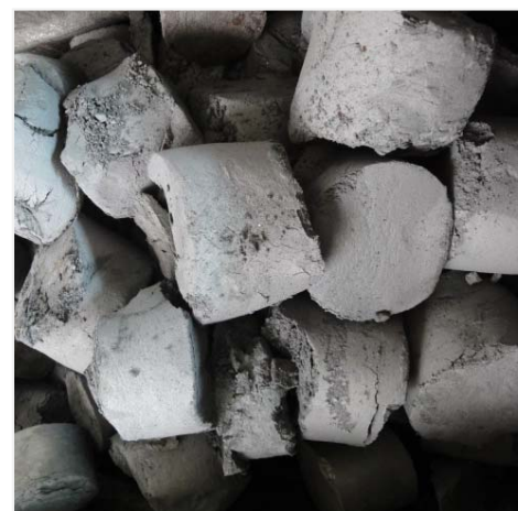
Picture 11-12: The pressing unit integrated into the MAXFLOW compresses the residues into briquets and ejects them into collection bins.
