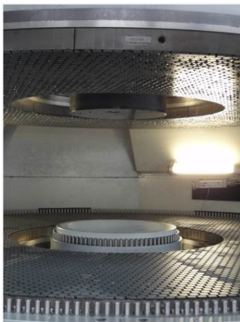
Picture 7: The Melchiorre ELC 2000 has grinding disks with a diameter of 2.000 millimetres.
