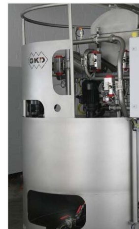
Picture 9: The compact filter of GKD combines filtration and briquetting in a single piece of equipment.
