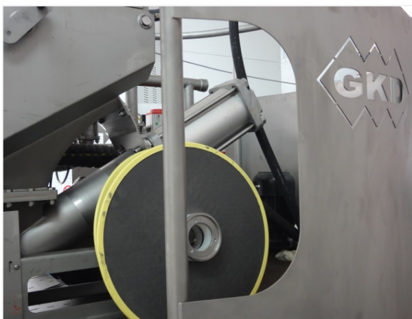
Picture 10: The filter head contains two filter packets each consisting of two vertically aligned static disc filters screened with YMAX® multidimensional blended filter mesh.
