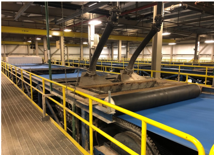
Picture 3: Phosphogypsum is dewatered on horizontal vacuum belt filters.
