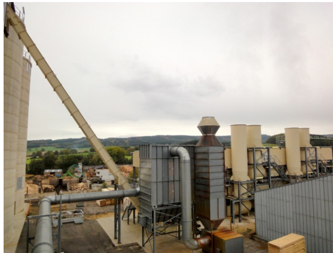
Picture 8: The wood chips produced are transported to the corresponding drying plants via an extensive pipe system.
