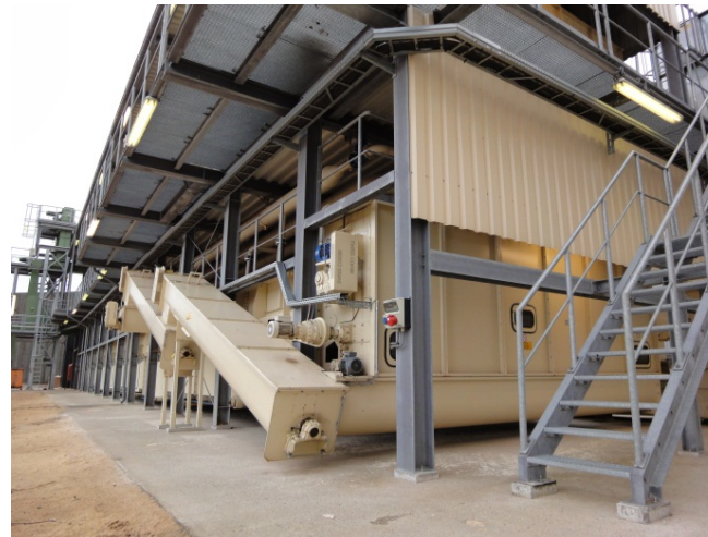
Picture 2: Low-emission, low-temperature belt dryers with process belts from GKD – Gebr. Kufferath AG.
