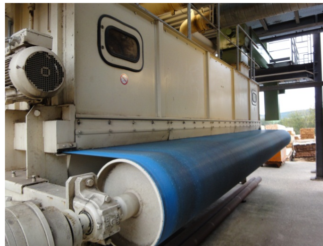
Picture 4: The endless permeable GKD mesh belt Conducto® 5065.
