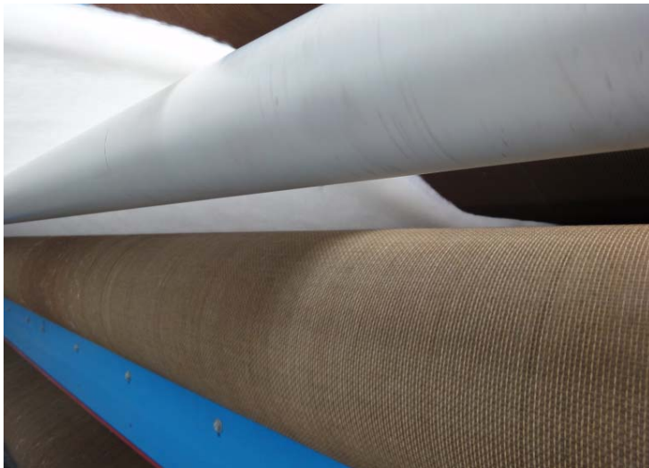
Picture 1: In exacting thermal bonding processes, the innovative anti-stick coated glass hybrid fabric belts from GKD offer much better process performance and product quality than glass gauze belts.
