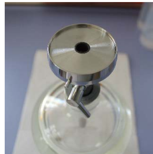
Picture 9: Base of the filtration apparatus with crucible. The crucible should be level.
