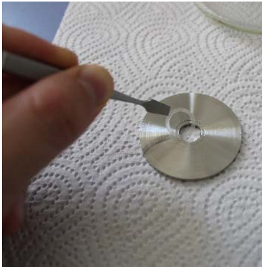
Picture 10: Insertion of the silicone sealing ring into the recess on the underside of the upper stainless steel disc. Applying pressure with the finger.
