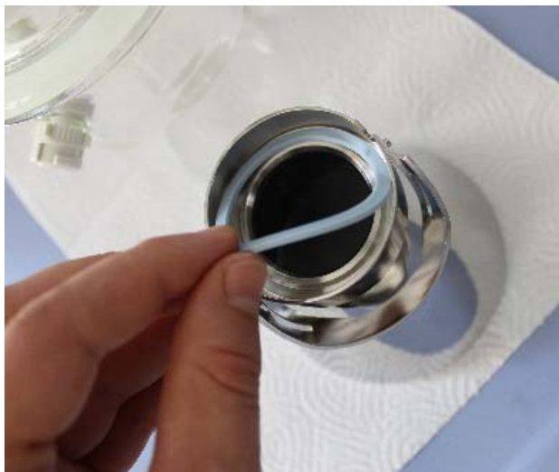
Picture 13: Insertion of the wide sealing ring into the recess at the bottom of the funnel (filtration attachment).
