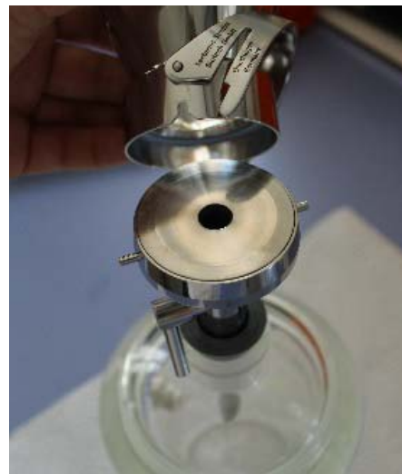
Picture 14: Placement of the filtration attachment straight onto the base, in the grooves provided.
