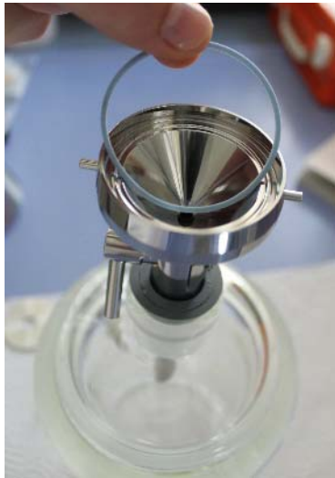
Picture 5: Inserting the narrow sealing ring into the stainless steel filtration apparatus.
