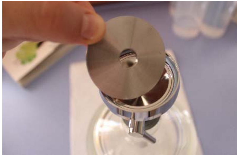
Picture 6: Insertion of the lower stainless steel disc; small graduation for the following crucible pointing upwards.
