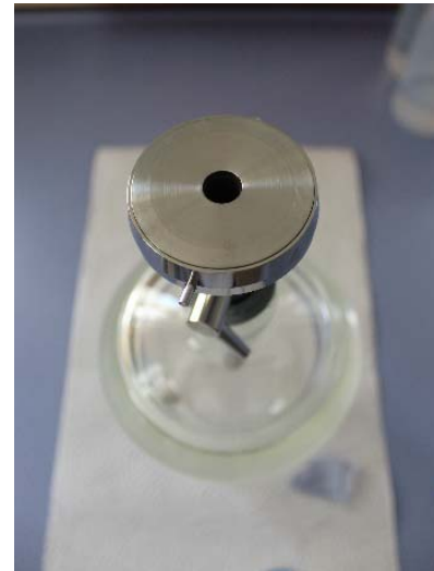
Picture 12: Base of the filtration apparatus with enclosed crucible.
