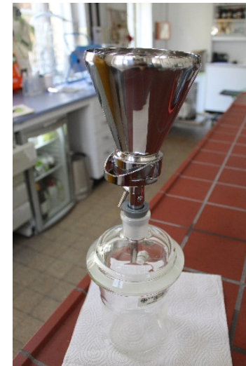
Picture 15: Sealing the filtration apparatus with the attached hook closure.
