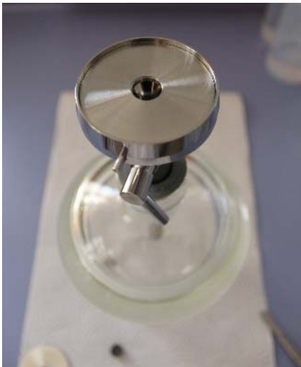
Picture 7: Base of the filtration apparatus without crucible.
