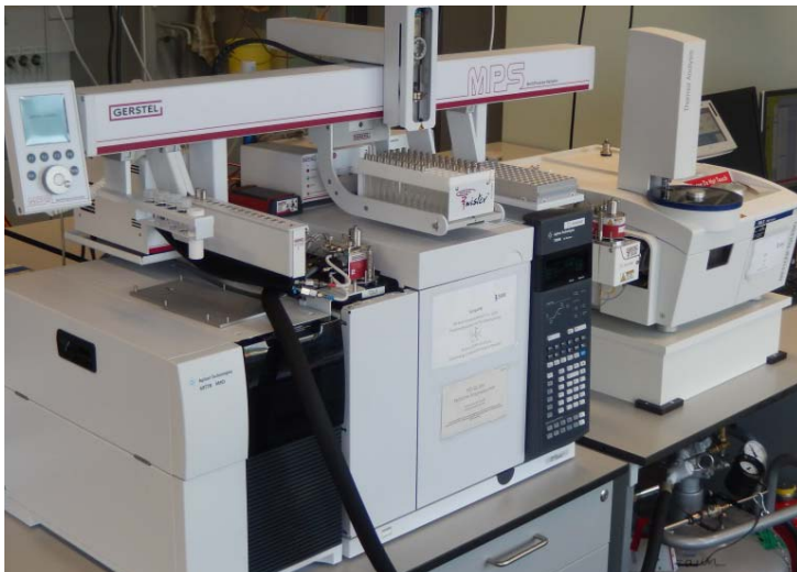
Picture 3: TED-GC/MS determines mass content in solid environmental samples both quickly and reliably.
