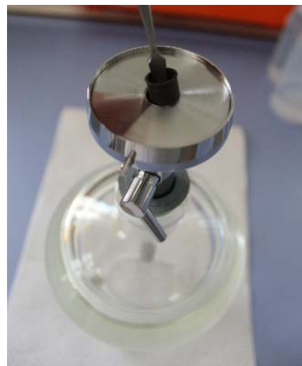
Picture 8: Insertion of the microlitre filter crucible into the hole of the lower stainless steel disc. The crucible rim should rest evenly in the small graduation.
