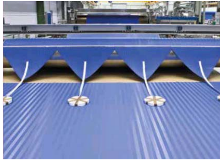
Picture 9: A specific unrolling function in the transport crates makes it possible for the heavy belt to be pulled into the machine directly from the crate with a special belt feeder and straps.
