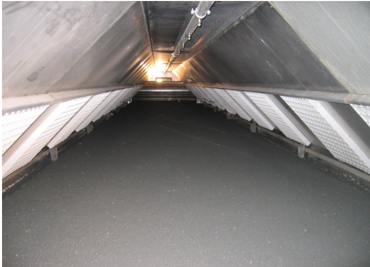
Picture 8: With air permeability optimally tailored to the drying process, the GKD 5099 PPC process belt ensures an efficient drying process despite the very closed surface.
