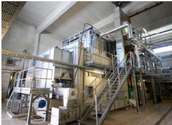
Picture 6: The belt dryer with a GKD 5099 PPC process belt has a drying capacity of 22,000 tons of wet sludge per year.
