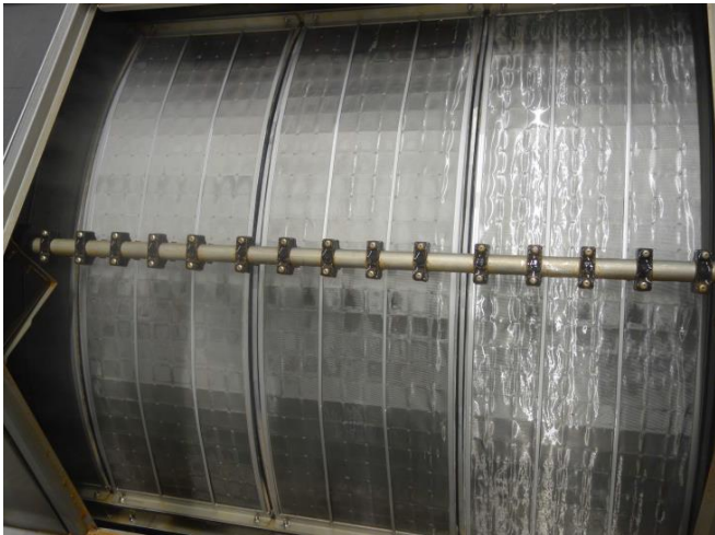
Picture 2: Porometric mesh from GKD proves itself in drum filters for mechanical water purification – as here in an indoor salmon farming facility at Swiss Alpine Fish AG.
