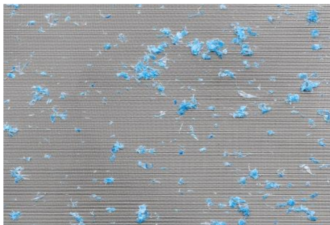
Image 2: Stainless steel Porometric mesh from GKD, with pore openings of 13 - 25 \mu\text{m} , is currently considered the best product on the market for water filtration.
